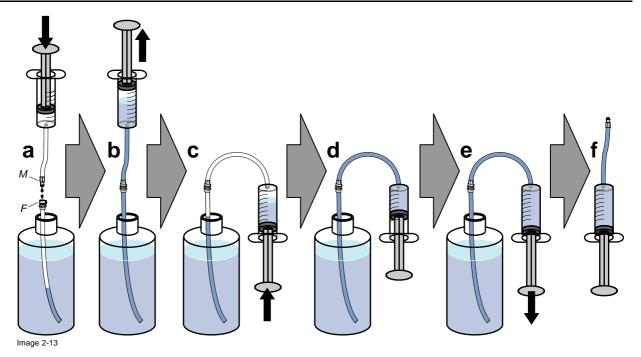
Couple the syringe to the inlet of the cooling circuit and press the cooling liquid inside the circuit until the manometer indicates 1 bar pressure. Ensure that no air bubbles are injected into the circuit.
